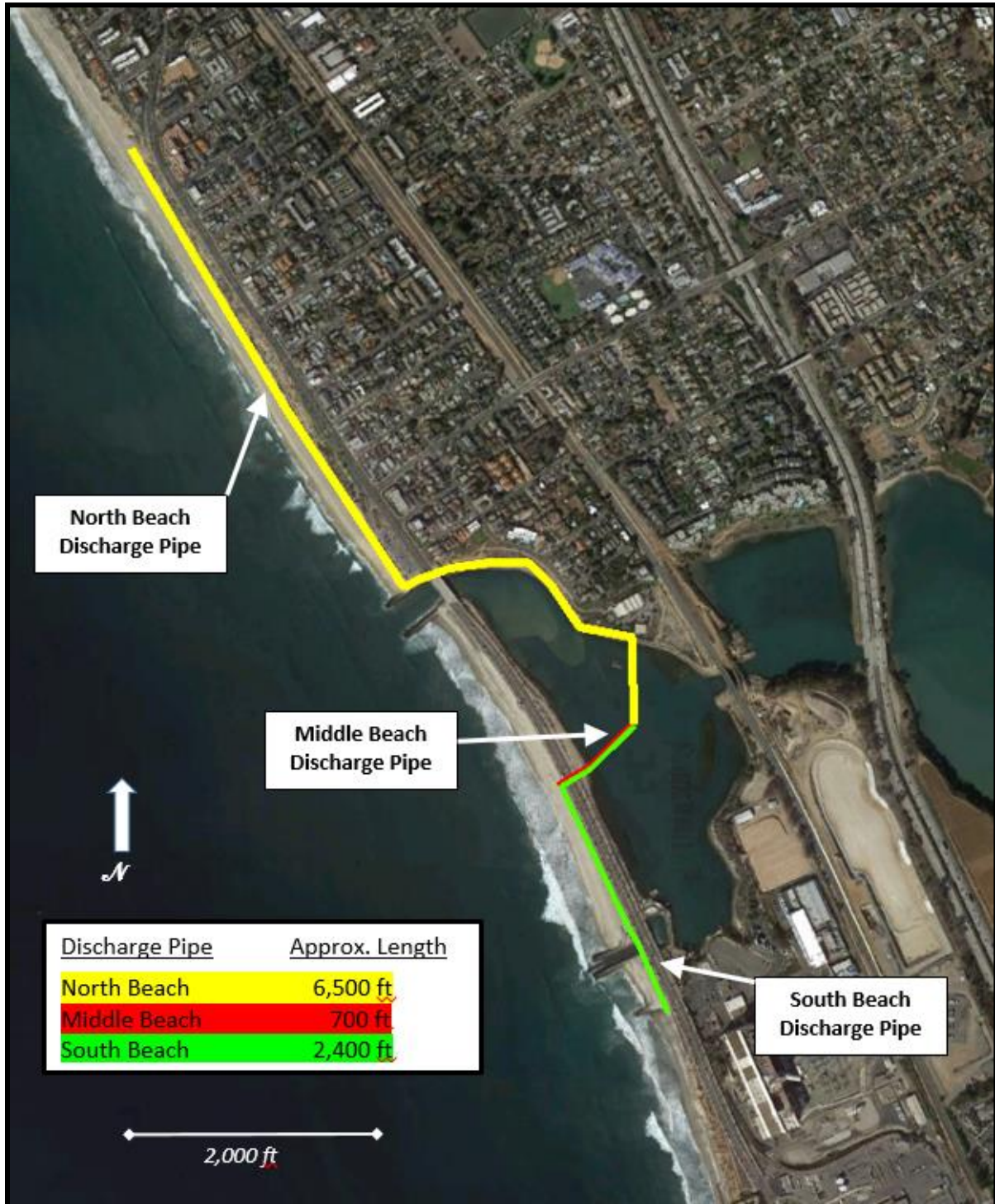
Figure 2. Dredge Discharge Pipeline Routes
