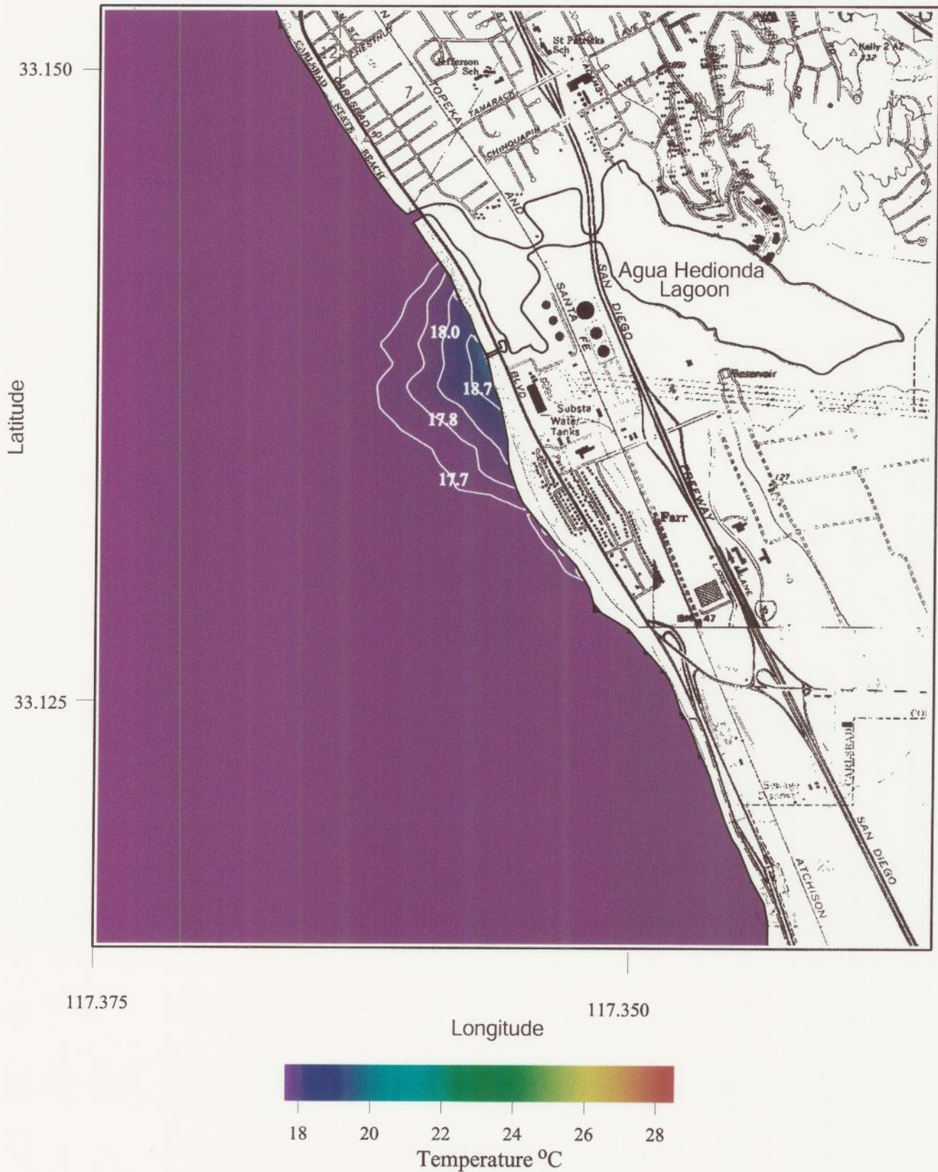
Figure 23. Historical average hydraulic case ( \Delta T = 5.5^\circ \text{C} ). Daily depth-averaged temperature of concentrated seawater for R.O. = 50 mgd, plant inflow rate = 576 mgd, combined discharge = 526 mgd, ambient ocean temperature = 17.6^\circ \text{C} , ocean conditions, 23 May 1994.
