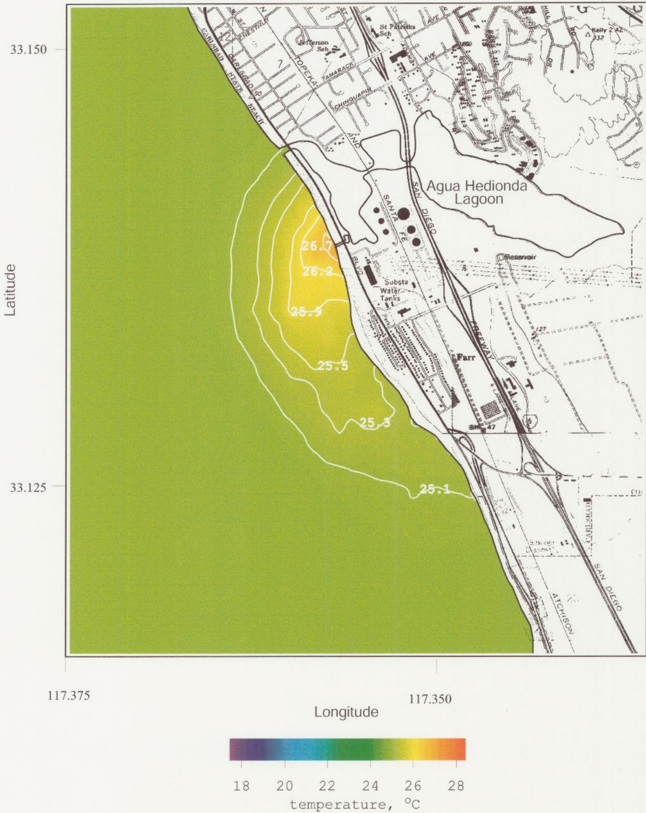
Figure 16. Historical extreme conditions for Unit 4 with 2 pumps, heated ( \Delta T = 5.5\text{ }^{\circ}\text{C} ). Daily average of the bottom temperature of concentrated seawater for R.O. = 50 mgd, plant inflow rate = 304 mgd, combined discharge=254 mgd, ambient ocean temperature = 25.0\text{ }^{\circ}\text{C} , ocean conditions, 17 Aug 1992.
