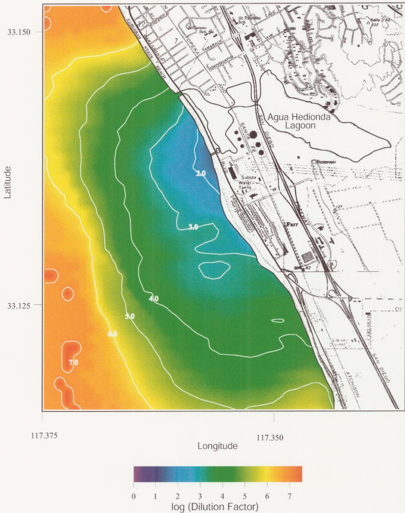
Figure 21. Historical average hydraulic case ( \Delta T = 5.5^{\circ} \text{C} ). Depth-averaged dilution factor for raw concentrate from desalination. R.O. = 50 mgd, plant inflow rate = 576 mgd, combined discharge = 526 mgd, ambient ocean salinity = 33.52 ppt, ocean conditions, 23 May 1994.
