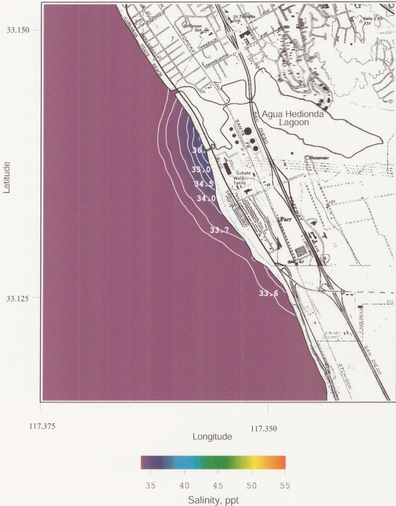
Figure 13. Historical extreme conditions for Unit 4 with 2 pumps, heated ( \Delta T = 5.5\text{ }^{\circ}\text{C} ). Daily depth-averaged bottom salinity of concentrated seawater for R.O. = 50 mgd, plant inflow rate = 304 mgd, combined discharge = 254 mgd, ambient ocean salinity = 33.51 ppt, ocean conditions, 17 Aug 1992.
