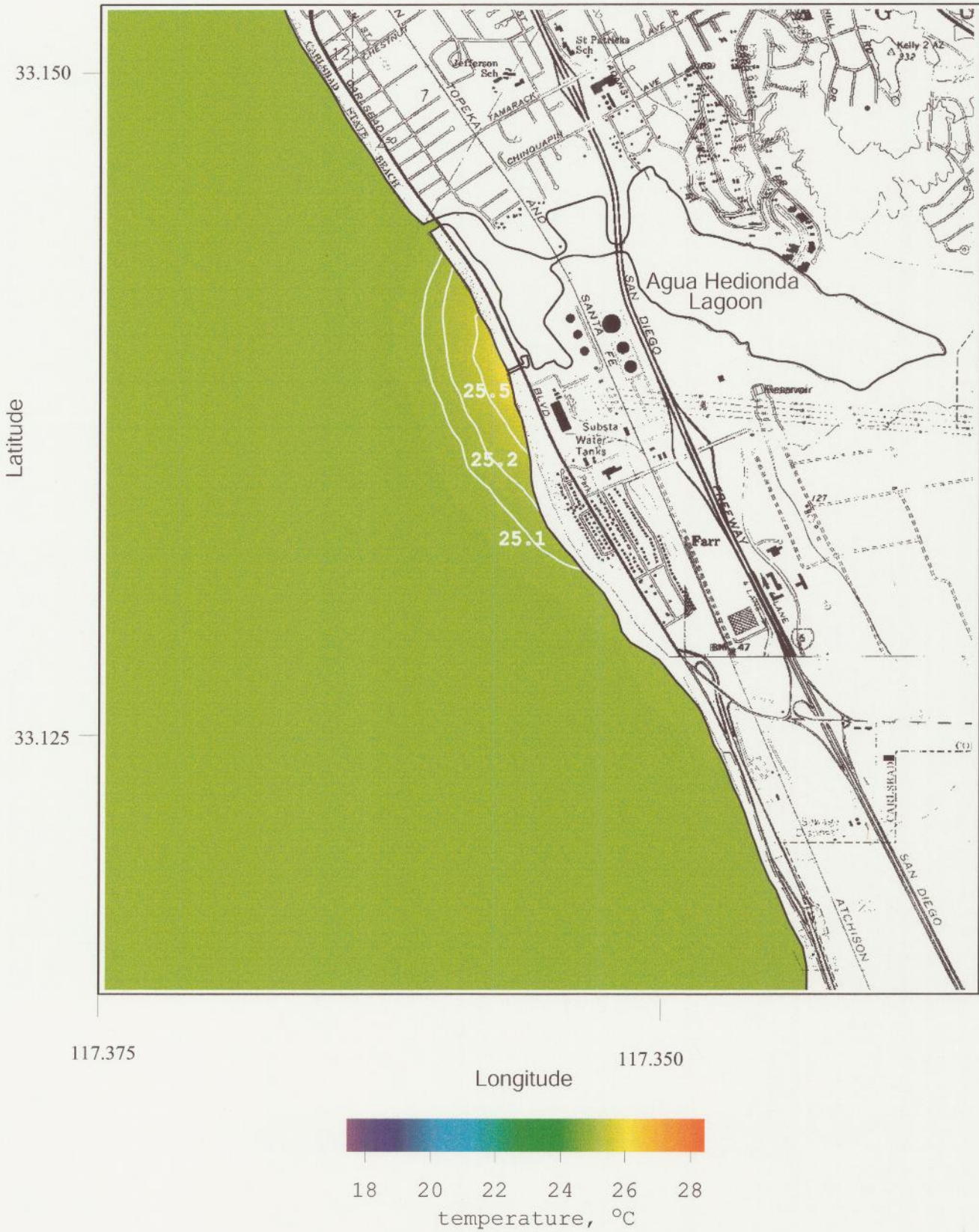
Figure 17. Historical extreme conditions for Unit 4 with 2 pumps, heated ( \Delta T = 5.5\text{ }^{\circ}\text{C} ). Daily depth-averaged temperature of concentrated seawater for R.O. = 50 mgd, plant inflow rate = 304 mgd, combined discharge=254 mgd, ambient ocean temperature = 25.0 ^{\circ}\text{C} , ocean conditions, 17 Aug 1992.
